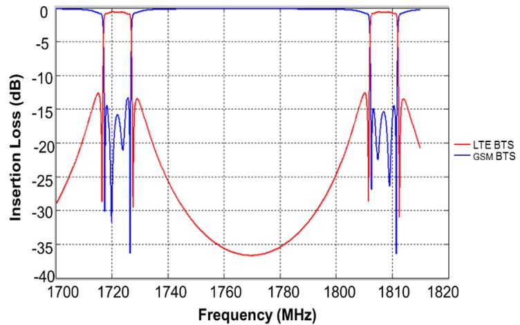
Figure 4. The LTE and GSM signals combined with ultra-narrow symmetrical guard bands
