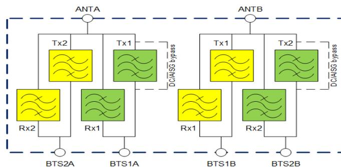
Figure 6. Dual MIMO In-band combiner
