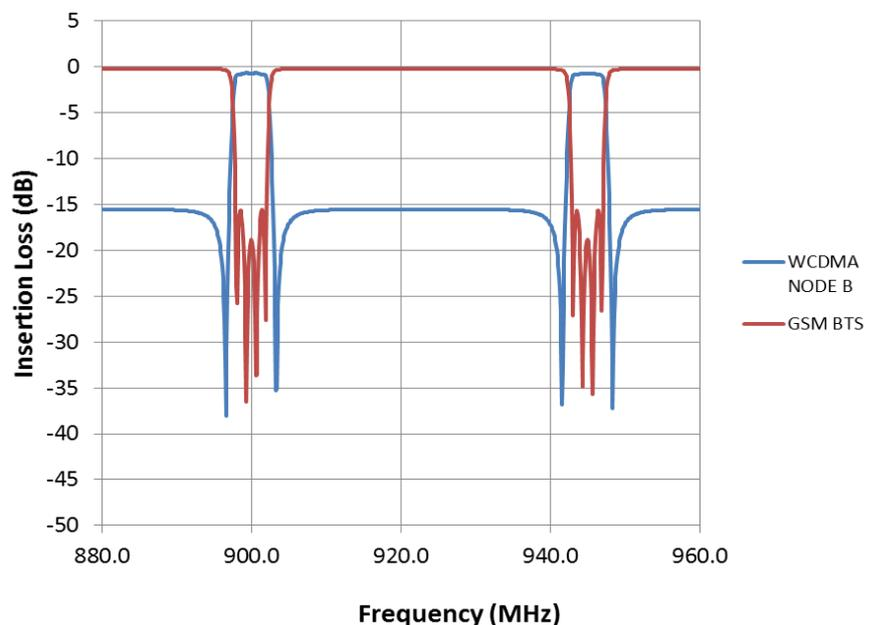
Figure 2. The WCDMA and GSM signals combined with very narrow symmetrical guard bands
