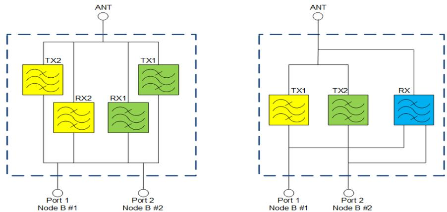
Figure 5. (a) The in-band combiner with TX and RX filters (b) The in-band combiner with TX filters and passive split RX
