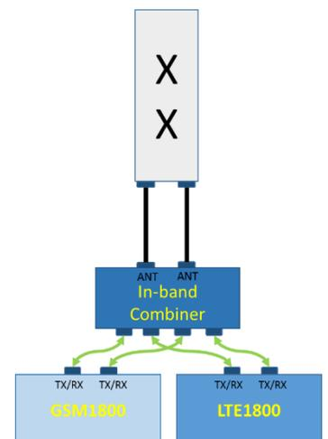
*Figure 1. The in-band combiner used to combine two signals within the same frequency band*
