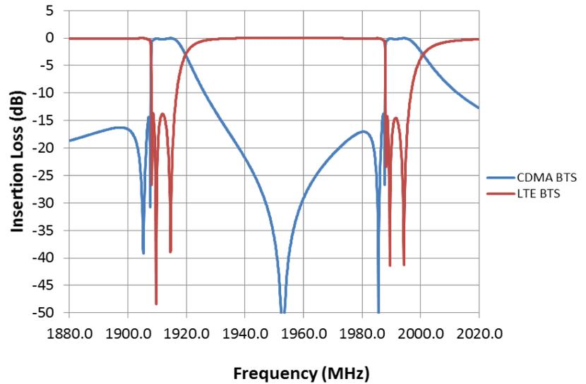
Figure 3. The CDMA and LTE signals combined with very narrow guard band
