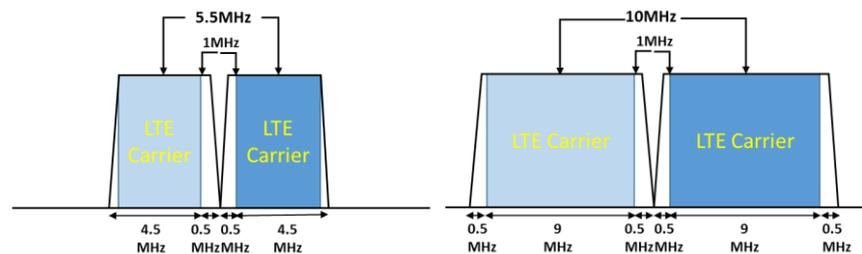
*Figure 7. Two continuous 5MHz and 10MHz LTE blocks combined with an In-band combiner with 1MHz guard band with no loss of spectrum*
